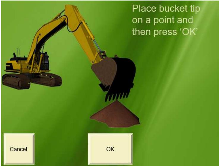
The swap point function is available for projects *“Flat plane”, “Single slope”* and *“Dual slope”*. Before you move the undercarriage, place the bucket tip on a point which can also be reached from the place you will be moving the undercarriage to. Press *“OK”* on the screen. Move the undercarriage and position the bucket tip on the same point. Press *“OK”* on the screen again.
