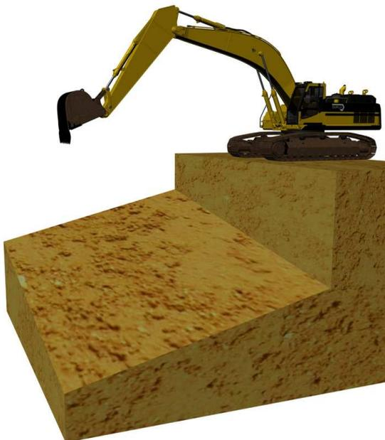
A dual slope is a surface with a gradient both lengthways and sideways. In DigPilot you need to set the following to work on dual slopes:
