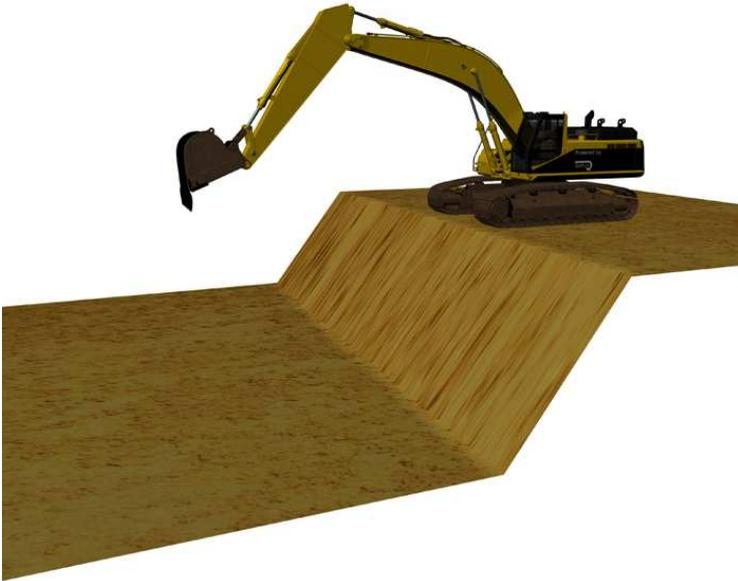
A profile consists of two horizontal surfaces of different height with a single slope between them. In DigPilot you need to set the following to work on a profile:
