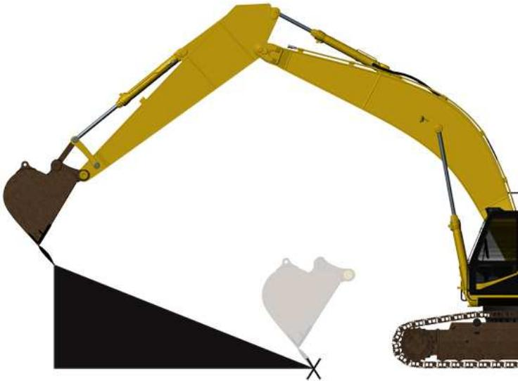
Bucket-defined is used to indicate a single slope using the bucket tip. This can be useful, for instance when forming a single slope up to the foundations of a garage.
