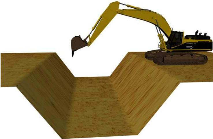
A channel consists of three horizontal surfaces with single slopes between them as shown on the illustration opposite, and has the same gradient on both sides of the channel base. With a channel the following settings must be entered:
